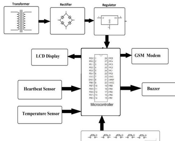
Fig. 1. Architecture of PHMS using GSM Module
