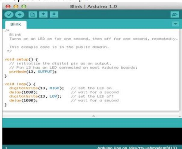
Fig. 5. Sample code for LED blink
