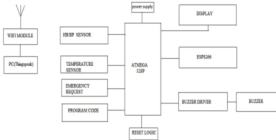
Fig. 2. IoT based Health Monitoring System using Arduino
